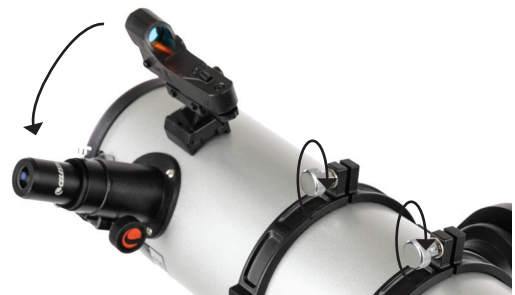
Figure 6a: To rotate the optical tube for a more ergonomic focuser position, simply loosen the clamping knob(s) on the tube rings or cradle.
